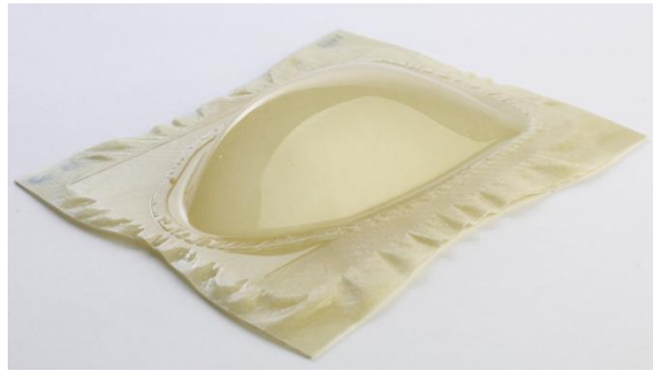
Fig. 7: Translucent StyLight* with glass fiber woven fabrics
